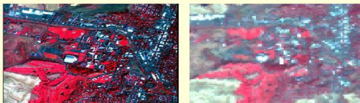
ESSI Inc Probe-1 Sensor Imagery: 5 x 5 meter spatial resolution Landsat 7 TM Imagery: 30 x 30 meter spatial resolution.
