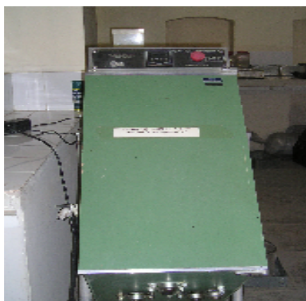
Mechanical Sieve Shaker
