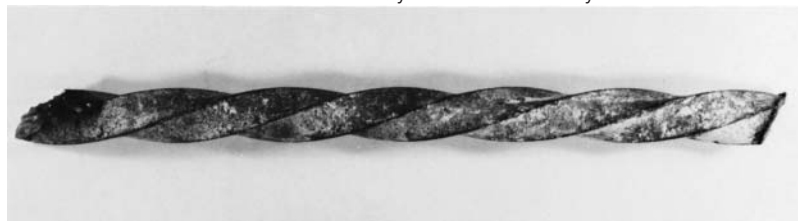
Twisted square bar, formerly used to increase bond between concrete and steel.
