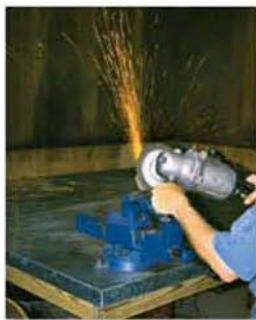
The heat generated by the abrasive action of friction can be noticed when using this grinder to sharpen a metal blade.
