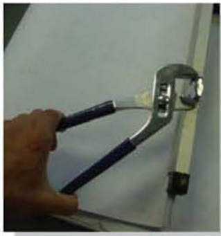
Common tools such as these pliers act as simple machines. Here the applied force on the handles creates a much larger force at the jaws.
