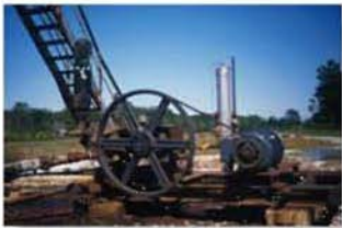
Flat or V-belts are often used to transmit the torque developed by a motor to a wheel attached to a pump, fan or blower.
