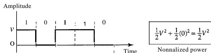
Figure 4.5 Unipolar NRZ scheme
