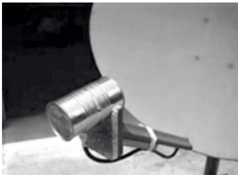
Figure 4.10: Feed horn made from a food can.
