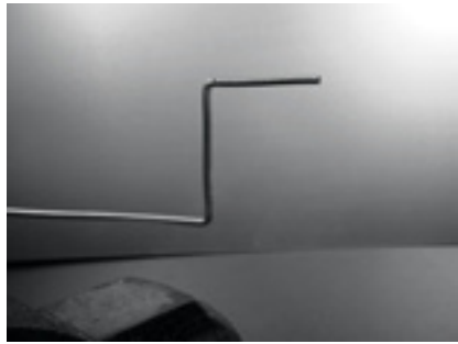
Figure 4.16: Bend the wire into a "Z" shape.
