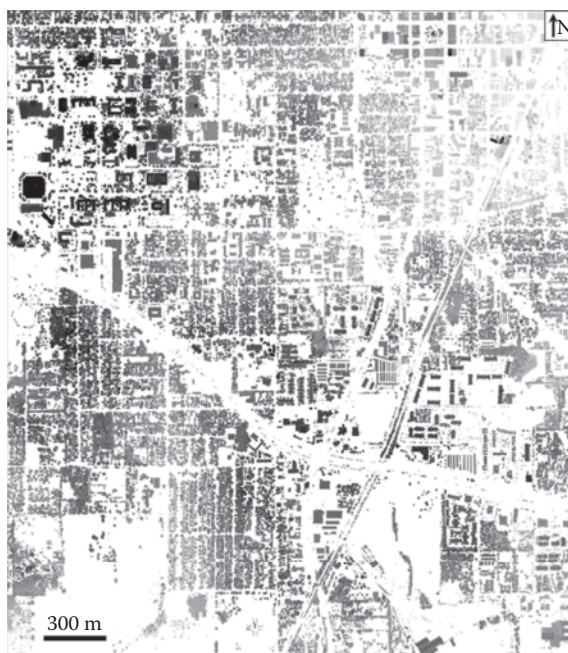
FIGURE 5.3 Non-ground DSM derived from LiDAR data.
